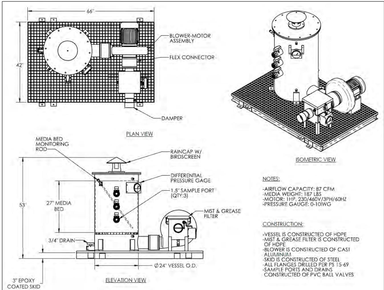
**Figure C-3** Vertical Air flow System Assembly
