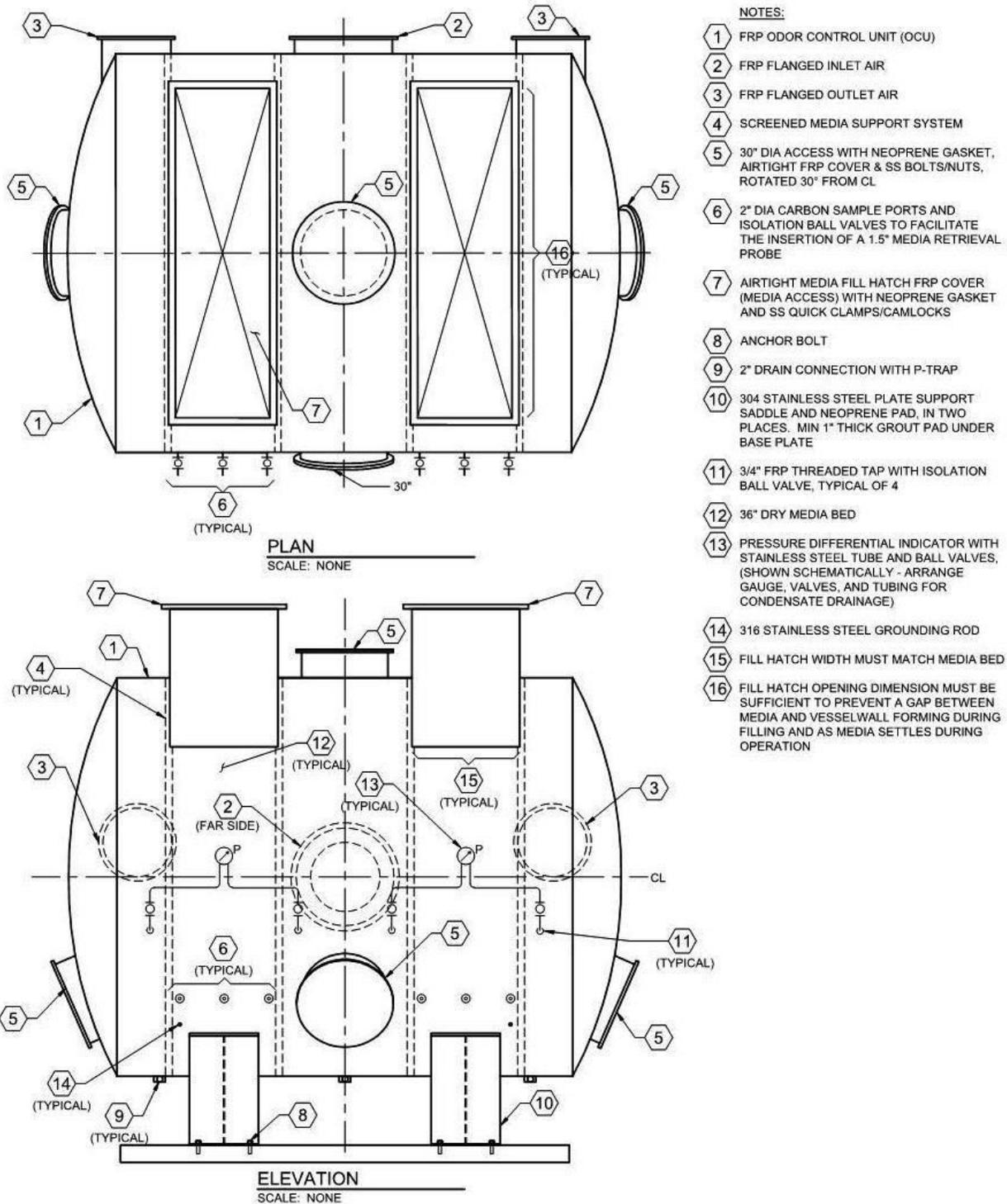
**Figure C-2. Typical Deep-Bed Dry Media Scrubber (Horizontal Air flow/Vertical Bed)**
