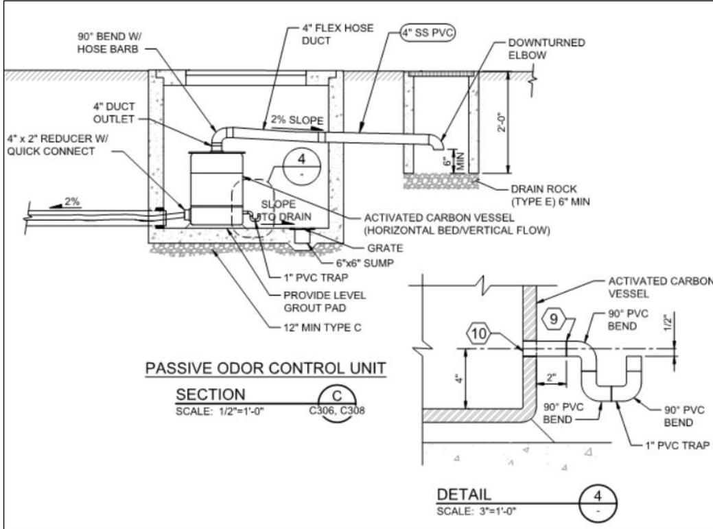
Figure C-5. Passive Air Release Valve Odor Control System
