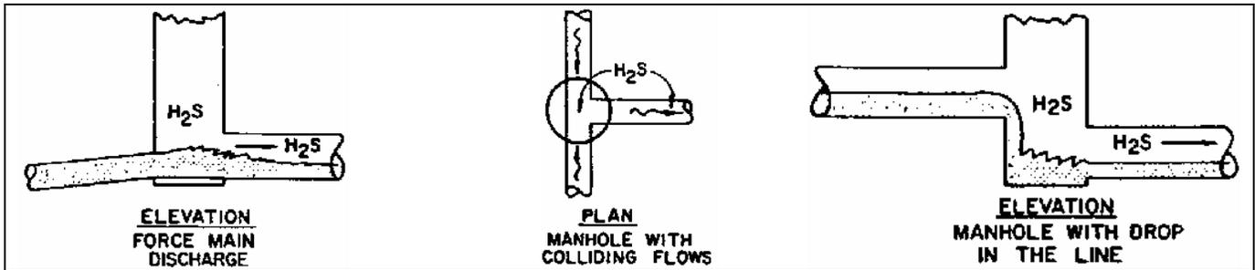
Figure 2. Sources of Turbulent Flow in Sewers
