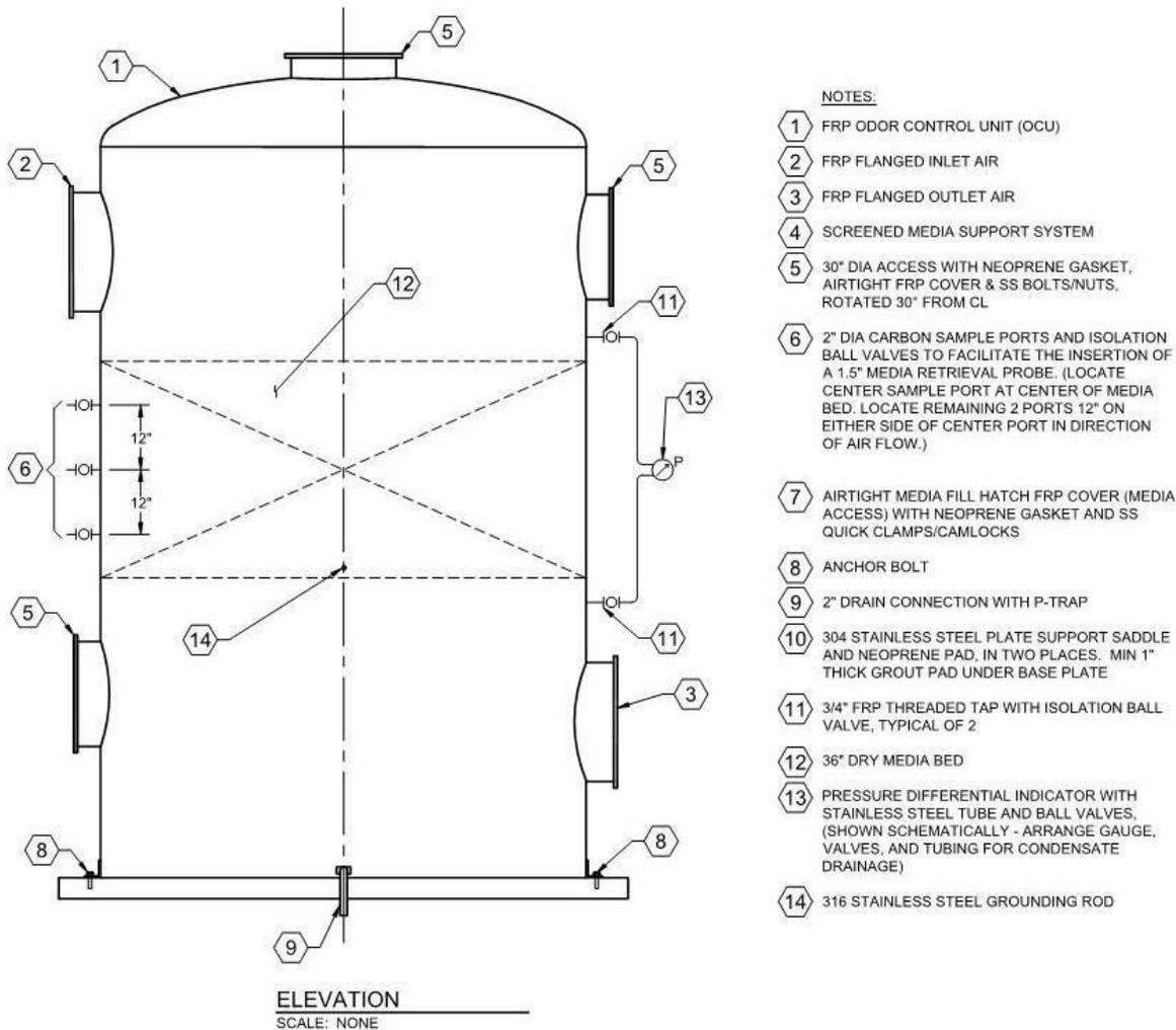
**Figure C-1. Vertical Air flow Deep-Bed Dry Media Scrubber**
