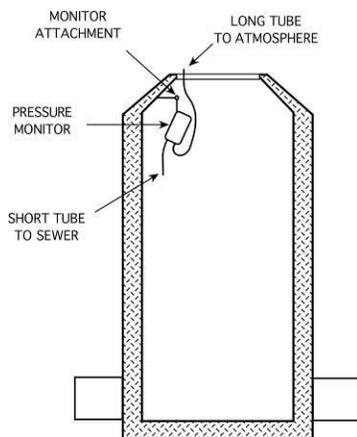
**Figure A-4.** Pressure Monitor Installation Diagram
